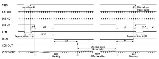
Fig. 16. Vertical timing for pulse width control 1/2 partial scanning
